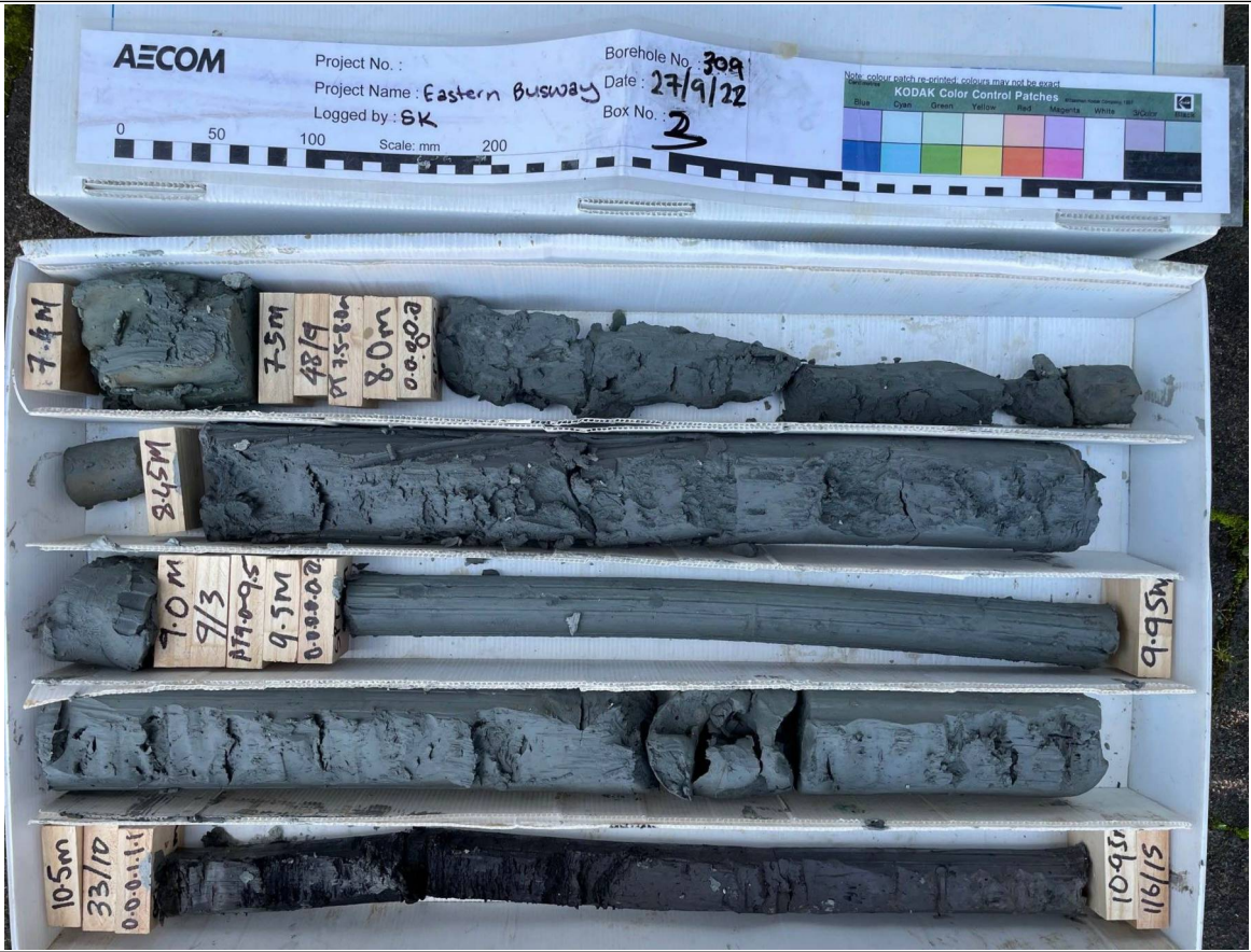
Box: 3 of 9 - Depth: P\DH309_P 07.40m to 10.95m of 30.00m Date Drilled 27/09/2022 to 29/09/2022 - Date Photographed: 27/09/2022
